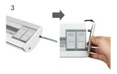
Using a Philips screwdriver (not included), untighten the screws and remove both end caps.
