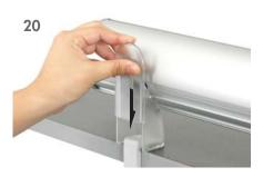
Slide stand cap onto the rear of the stand. Push down and snap into place.  $\,$
