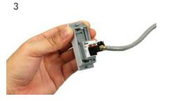
Terminate cable to keystone jack (refer to "Technical Specifications" for recommended jacks) and attach jack to data socket housing. If in doubt, consult a qualified electrician/installer.
