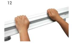
Align the track to the backplate and snap onto the main housing.
