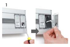
Using a screwdriver, detach data socket housings from the main housing.
